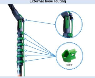
Fit hose clips NLHKP into the clips of the nLITE telescopic pole. Guide the hose through the clips on the outside of the pole and connect it to the angle adapter using the quick connector on the angle adapter.
